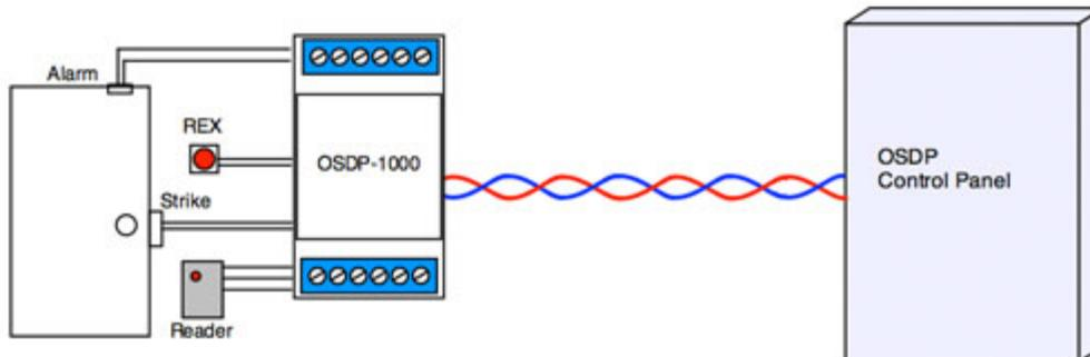
**Credential Reader** - Any Wiegand (Data 0 / Data 1), Strobed (Clock/Data), F/2F, or Serial interface can be handled by the OSDP-1000 when configured in "Reader Interface Mode". Since the format of the data is reported by the OSDP-1000 to the new control panel as an array of bits or characters, the panel's software must be configured to process the raw bit stream or character string. The reader type is configured by either on-board DIP switch or via OSDP configuration command from the panel.
