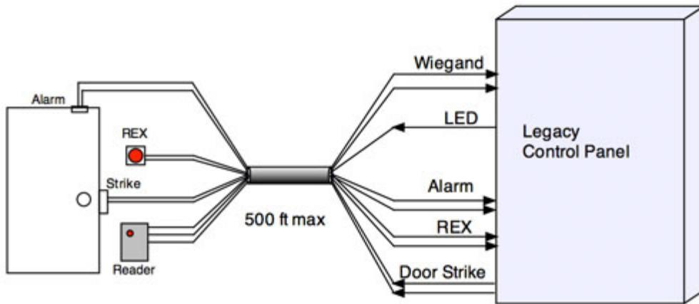
When the need arises to replace or upgrade a card access or security control panel and if the new panel is OSDP compliant, it may be advantageous or necessary to convert the field devices to OSDP compatibility. This normally means replacing all readers, sensors, contacts, relays, and door control equipment to OSDP compliant versions as well. If this is not an immediate option due to time or cost constraints, the Cypress OSDP-1000 can provide an effective solution.
